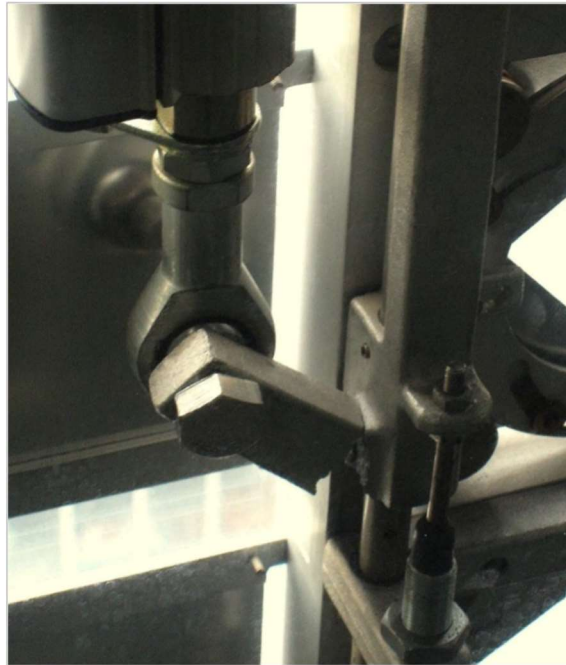
Figure 2.12: Damage on the motor force transmitting arm of the diaphragm actuation mechanism
